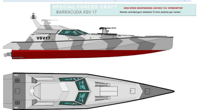
stealth aspect, into a usable practicable vessel by utilization of uniquely developed movable outer skin structures. These unique features work together with RAM and specialized outfitting, including minimal metallic fittings above decks. All of which combine to produce a vessel with a very significantly lower than normal RCS from all aspects.
